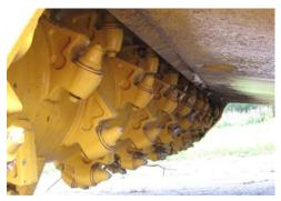
**UNT rotor C/W** special conical tips have extra indepth carbide, work ideally at low rotor speed.
