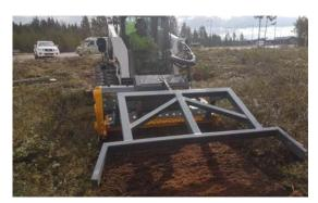
**Optional hydraulic push bar** is used for felling trees and directing tall material
