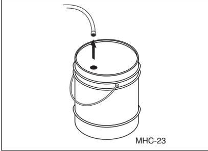
**STEP 1:** Remove detergent suction tube from container and insert into one (1) gallon of fresh water. Pull trigger on spray gun and siphon water for one minute.
